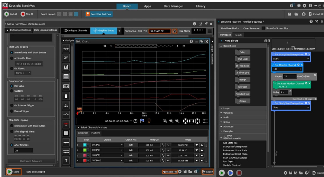
Figure 7. Example of Keysight's PathWave BenchVue data acquisition application software, which runs from a PC to configure and visualize data and export results
