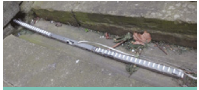
Image 3 A reconfigurable robot inspecting drains
