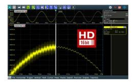
The Rohde & Schwarz RTx-K31software option provides essential measurement functions for analyzing power electronics, including inrush current, output spectrum and safe operating area. A measurement wizard with detailed instructions guides the user through the test setup. The oscilloscope configures itself automatically and delivers quick results.Optimal display configuration for each task.
