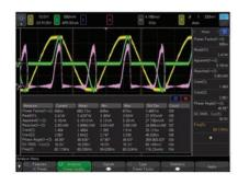
The Keysight DSOX6PWR is a power measurement and analysis option integrated into InfiniiVision 6000 X-Series scopes. The embedded application provides a quick and easy way of analyzing the reliability, efficiency and performance of your switching and linear power supplies.
