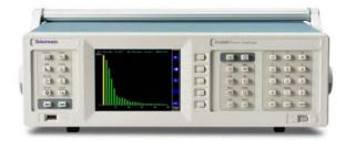
The Tektronix PA3000 is a one-to-four-channel power analyzer that is optimized for testing today's single and multi-phase, high efficiency power conversion products and designs. Use it to quickly visualize, analyze and document power efficiency, energy consumption, and electrical performance to the latest regional and international standards, including Level VI, EnergyStar, CEC, IEC 62301, CQC-3146 and more.
